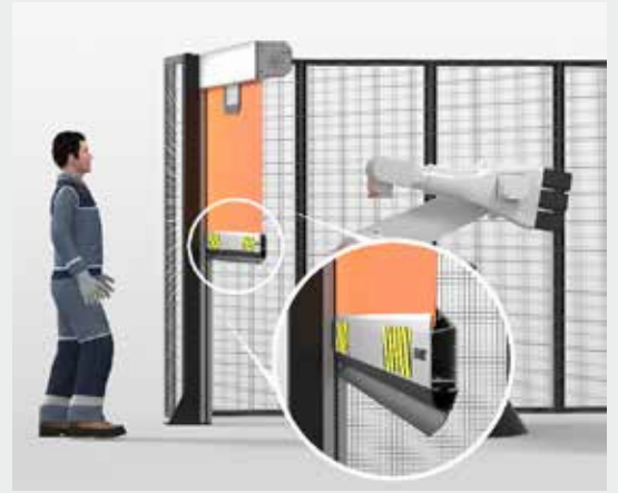
Version B* Flat side of the profile faces back side of the door
